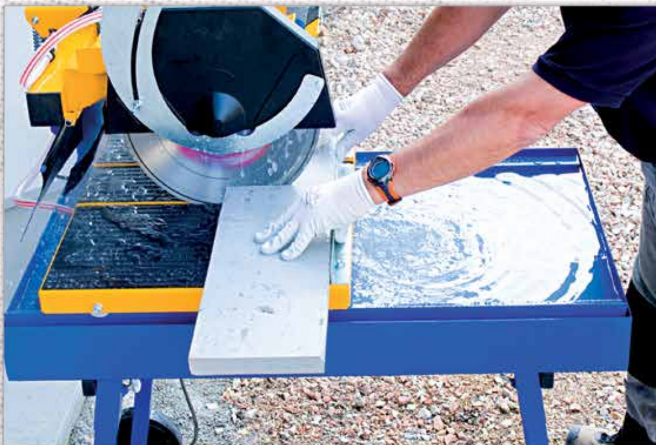
TAGLIERINA DA CANTIERE / FRESA A PONTE MASONRY BENCH SAW MACHINE / BRIDGE SAW
