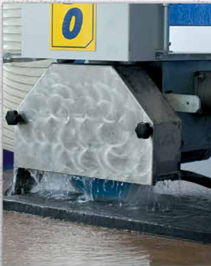
TAGLIERINA DA CANTIERE / FRESA A PONTE MASONRY BENCH SAW MACHINE / BRIDGE SAW
