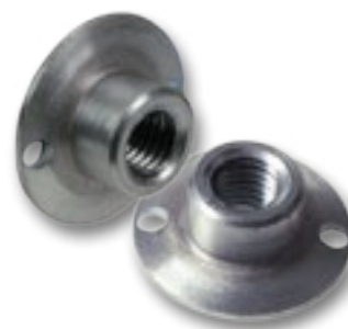
CONE-SHAPED RING NUTS W/LONG THREADED NECK Cone-shaped ring nuts with MA14 long threaded neck, for use on hand grinders (for holding flexible and semi-rigid carbide discs)
